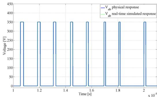
(b) Zoom-in of line-to-line voltage  $v_{ab}$
