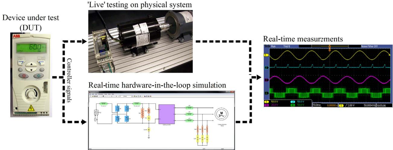
Fig. 1. A demonstration of a hardware-in-the-loop simulator (bottom) emulating the exact response of a physical system (top) in real time.
