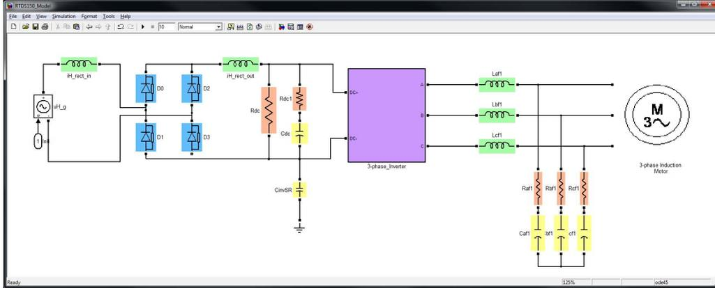
Fig. 2. A sample power electronics system described in the flexible schematic editor. From here the generation of real-time models of power electronics is completely automated.
