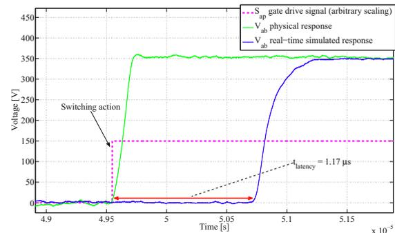
Fig. 3. A three-phase inverter line-to-line voltage response to a gate drive signal. Latency on the order of  $1\mu\text{s}$  is demonstrated by the real-time digital simulation.
