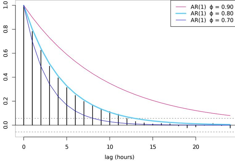
Figure 4: Autocorrelation of day-ahead forecast errors from the Grand Maison wind farm, compared with the theoretical autocorrelation (8) of an AR(1) model for three different values of the correlation coefficient  $\phi$ .
