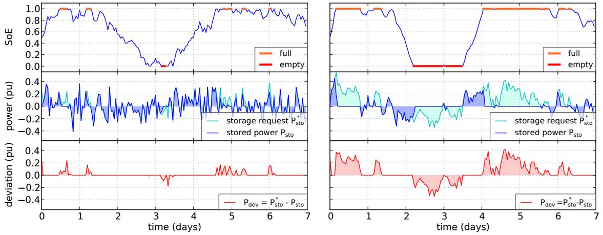
Figure 6: Stochastic simulation of an ESS, with two different correlation values for the autoregressive input model:  $\phi = 0$  on the left while  $\phi = 0.80$  on the right. In both cases,  $\sigma_P = 0.16$  pu and  $E_{rated}^{norm} = 15$
