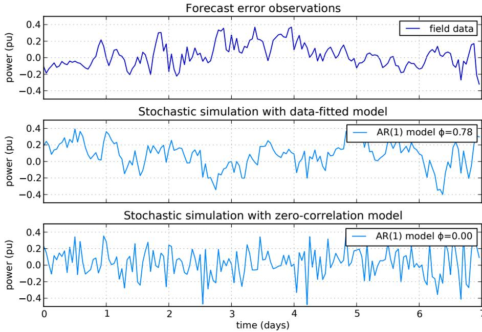
Figure 5: Comparison between forecast error  $P_{sto}^*$  from field observations and two stochastic simulations (AR(1) model with  $\sigma_P = 0.16$  in both cases while  $\phi = 0.78$  and  $\phi = 0$ , in the middle and bottom panels respectively)
