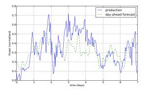
We focus on the difference between production and forecast because  $P_{sto}^*$  is the input of the storage control.
